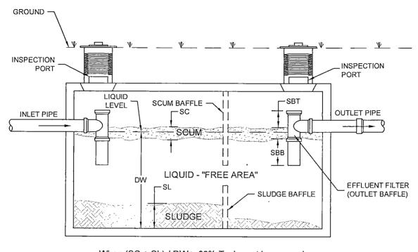
When (SC + SL) / DW > 33% Tank must be pumped. example (8" + 12") / 44" = 45%
